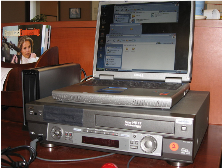
Figure 3: HPATV Ingest Station 2, Primarily Digital Files and DVD's
