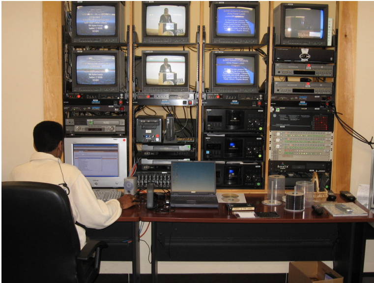
Figure 5: Believe it or not, this is HPATV's complete 4-channel playback facility after converting to full digital playout
